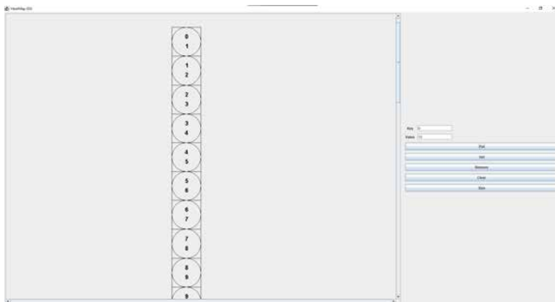
Fig. 8. Doubling the size when reaching 75% capacity
